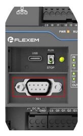
串行通讯接口 1 为 DB9 型式,支持 RS485 或者 RS232 通讯,引脚定义如下。Serial communication port 1 is DB9 type and supports RS485 or RS232 communication with the pin definitions as follows.
